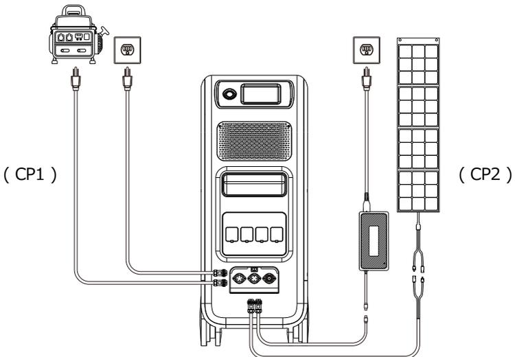
**Charging Method 5:** The EP500 supports charging with CP1 and CP2 at the same time. You can use any charging methods previously listed, simultaneously, to maximize your charging power input. They are listed here again for your convenience. Select one method for CP1 and one method for CP2 for simultaneous charging.
