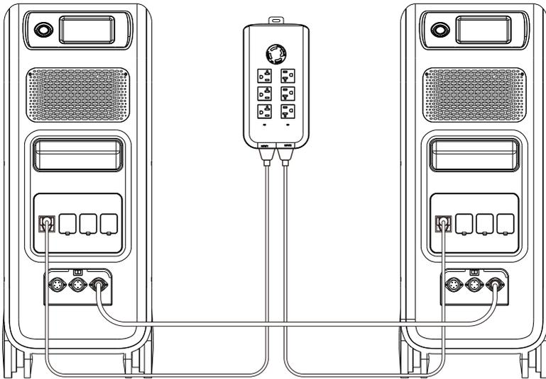
“Single Phase” is set as the default machine type if you are operating a single EP500. This is the only and correct setting if a single EP500 is being used. Machine type is used to enable "Split Phase". Split Phase is used for connecting two EP500 units (exclusive for the 100-120V version) by bonding them effectively into one larger power system to double the output power, voltage, and capacity. Please refer to the Split Phase setting section for more detailed information.
